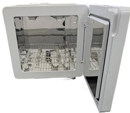
Fig. 3: UV-C light chamber with reflectors
