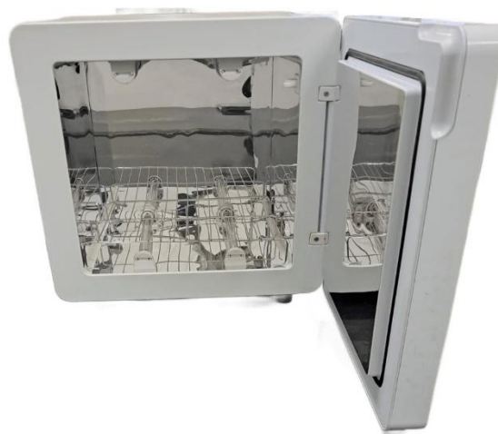
Fig. 3: UV-C light chamber with reflectors
