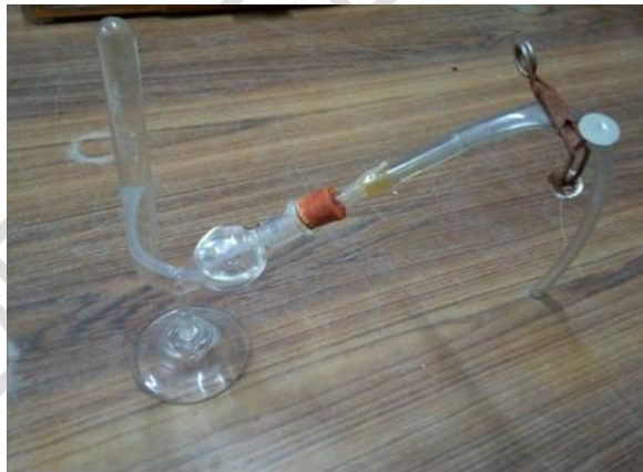
Measuring Biogas Methane content using Saccharometer
