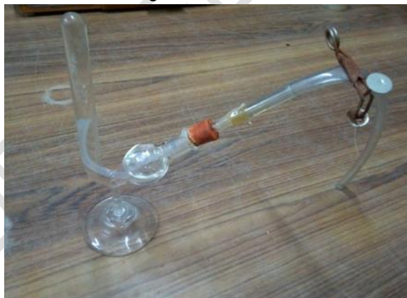
Measuring Biogas Methane content using Saccharometer
