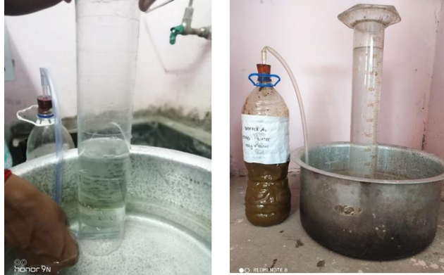
Water displacement method - Biogas volume measurement
