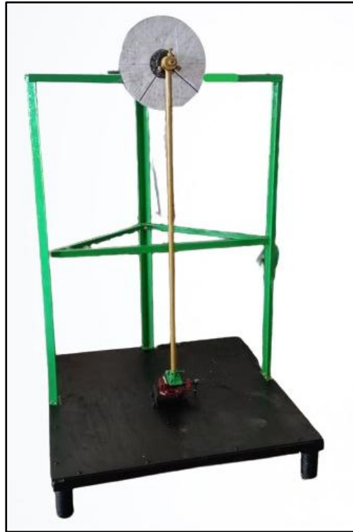
Fig.3.(write as Figure 3:) Developed pendulum impact cutter
