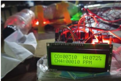
Figure 13 : Test results on LCD display
