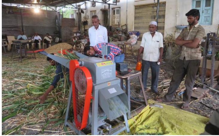
Fig.7:Performance of power operated chaff cutter
