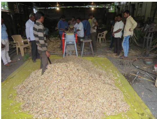
Fig.6: Performance of a power-operated chaff cutter for wet and dry fodder
