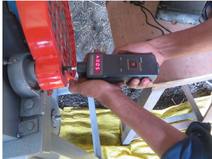
Fig.5: Measurement of the speed of the prime mover, cylinder, and feed roller using a digital tachometer during no load and load conditions
