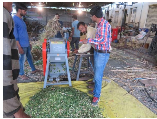
Fig.6: Performance of a power-operated chaff cutter for wet and dry fodder
