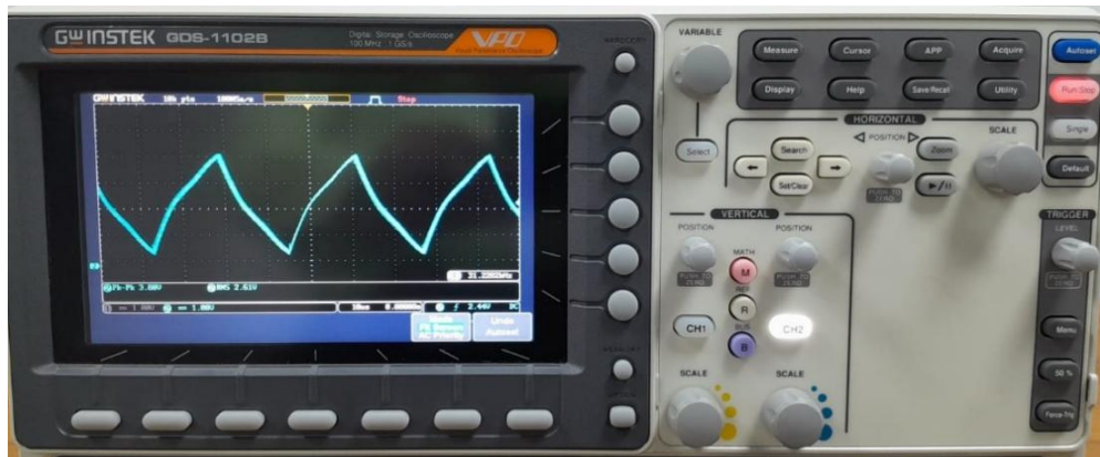
Fig. 12. Generated signal frequency on the digital storage oscilloscope screen.
