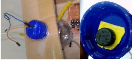
Figure 9 : Sampling box and RS1101 inside the blue cap
