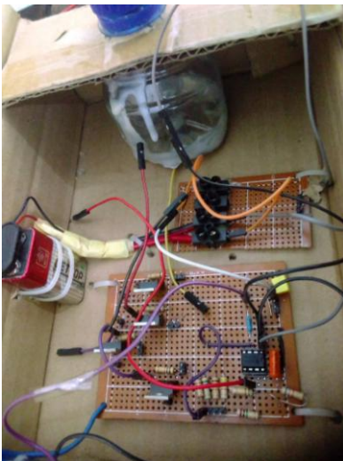
Figure 8 : Prototype with sampling box
