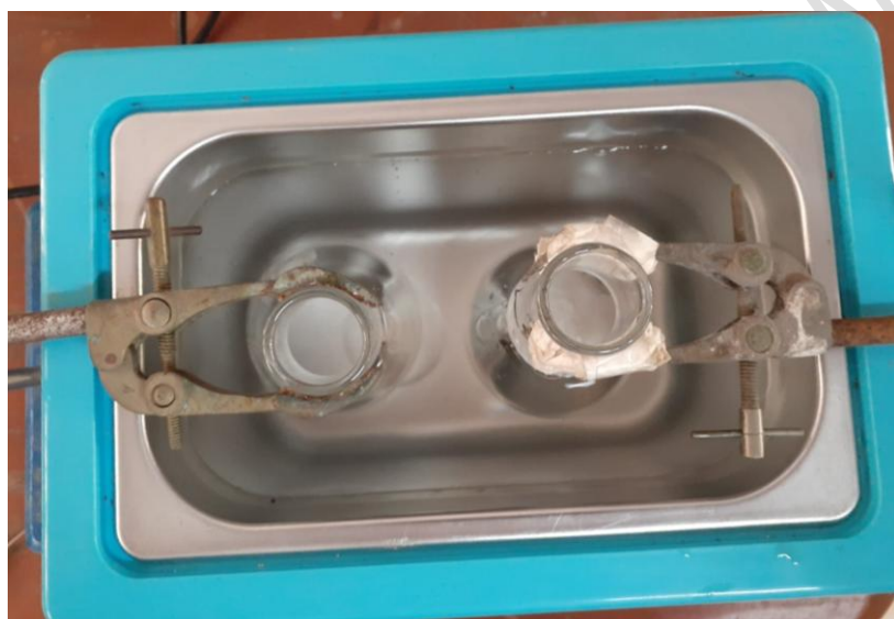
Fig. 1: Sonicator bath used in sonochemical degradation. ( formatting merge figure 1 and 2 )
