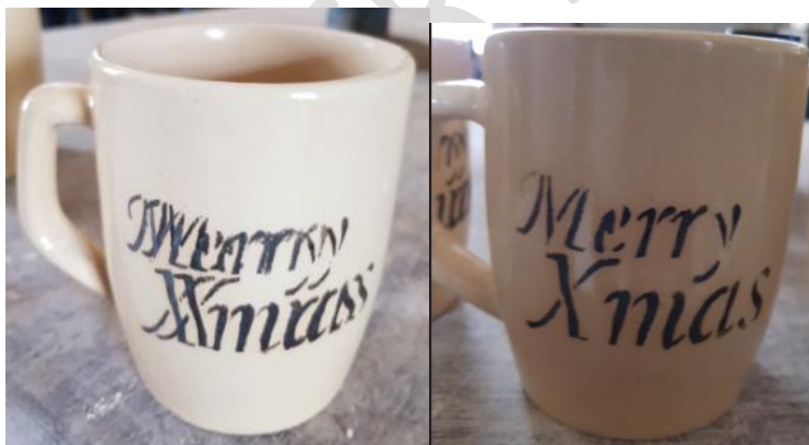
Fig. 4: Enamels from bone ash (left) and tin oxide (right) print on ceramic cups
