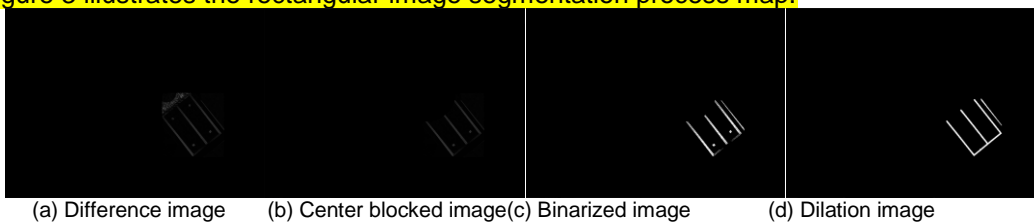
143 144 (a) Difference image (b) Center blocked image(c) Binarized image (d) Dilation image 145 Figure3 Rectangular target segmentation process
