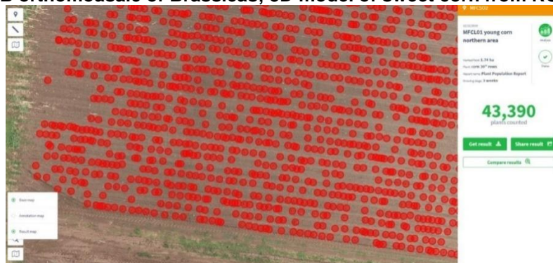
Fig. 4: Automated Plant Counts in Sweet Corn. Red circles indicate counted plants
