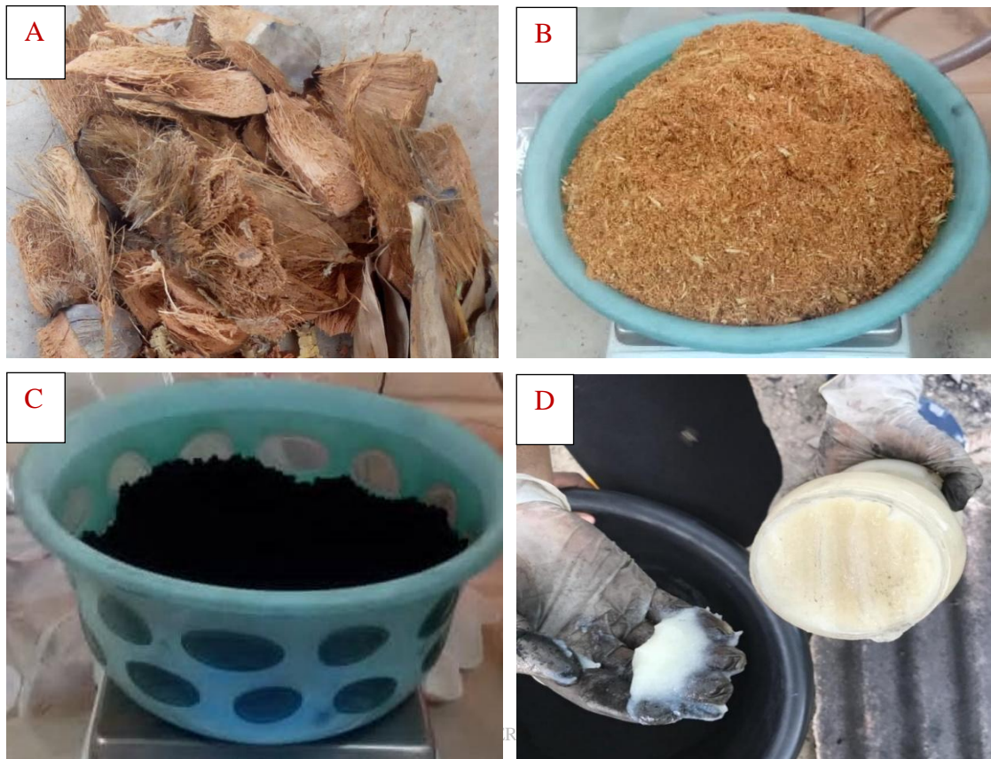
Figure 1: Biomass feedstocks used as raw materials (A) Coconut husk (B) Sawdust (C) Charcoal particles and (D) Cassava starch as binding agent
