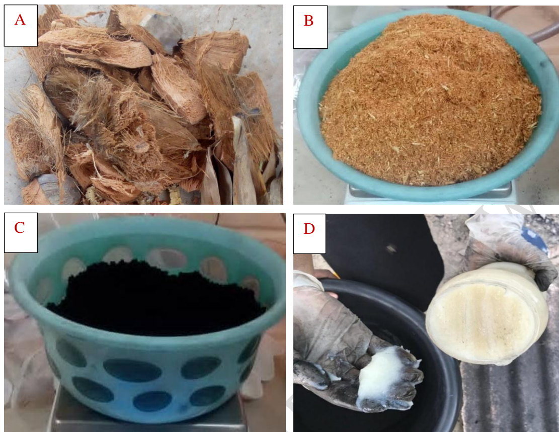
Fig. 1. Biomass feedstocks used as raw materials (A) Coconut husk (B) Saw dust (C) Charcoal particles and (D) Cassava starch as binding agent
