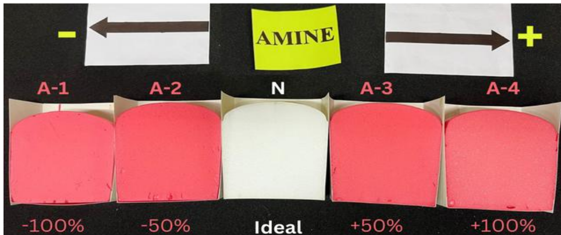
Fig. 6b: A visual illustration of the impact of varying amine concentrations on the quality of eventual flexible polyurethane foams.
