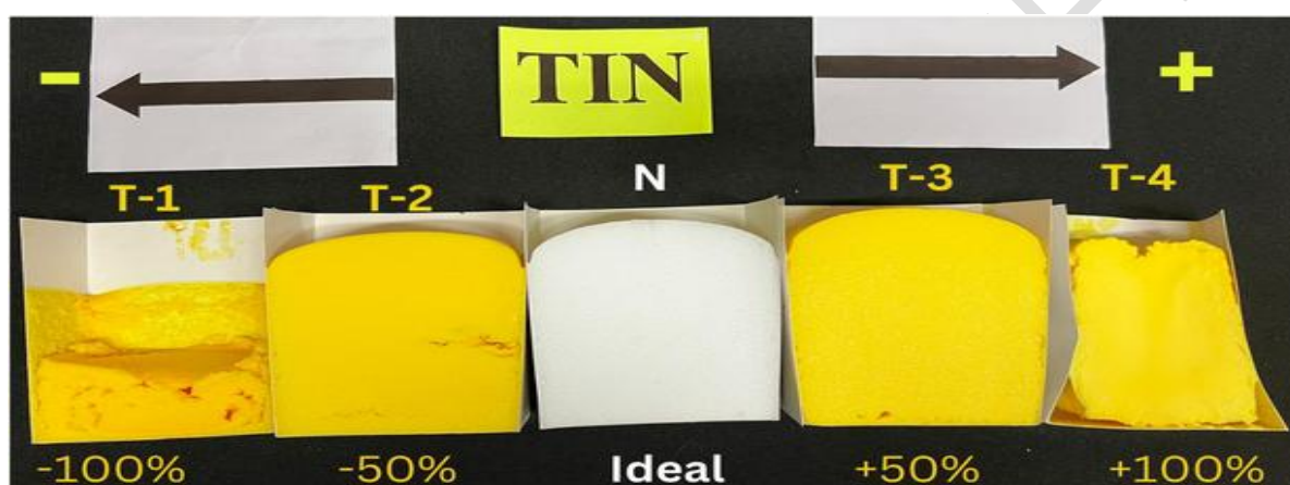
Fig. 5b: A visual illustration of the impact of varying stannous octoate (tin) concentrations on the quality of eventual flexible polyurethane foams
