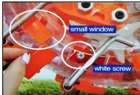
Fig. 2: Adjust the plant spacing
