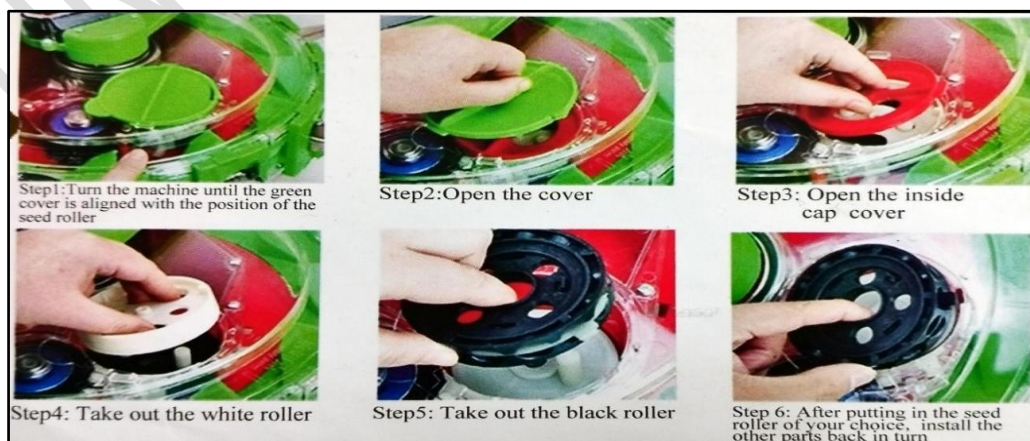
Fig. 3: Change the suitable seed roller
