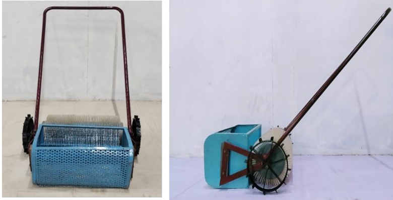
Fig.5. Mechanical type neem fruit picker collector
