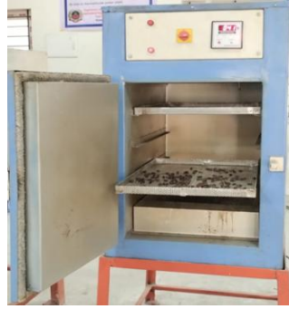
Fig.2. Measurement of moisture content of neem fruits using hot air oven
