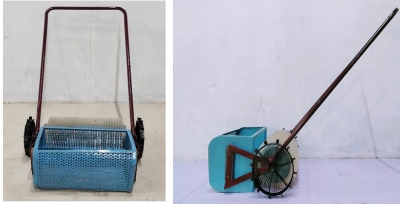
Fig.5. Mechanical type neem fruit picker collector
