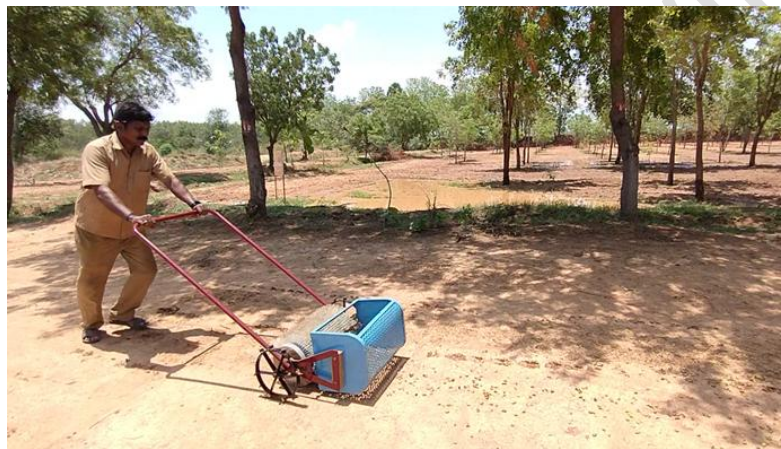
Fig.6. Operation of neem fruit collection using the developed prototype
