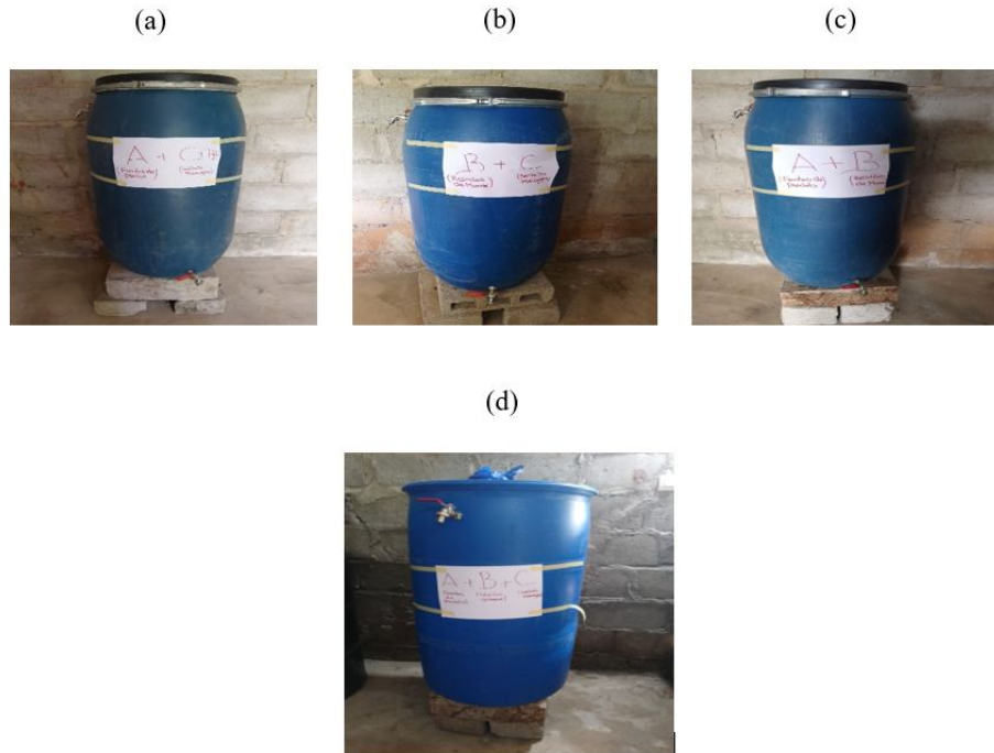
Fig. 2. The 160 liter and 200 liter digesters: (a) 160 liter digester 1, (b) 160 liter digester 2, (c) 160 liter digester 3 and (d) 200 liter digester 4
