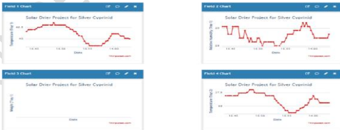
Figure7:Data recording and tracking using ThingSpeak Matlab Extension.
