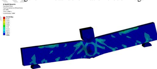
FIG. 13 Equivalent stress cloud image
