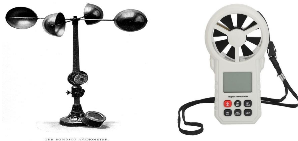
Fig. 4. A cup and a hand-held anemometer
