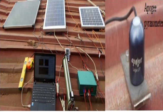
Figure 5. Experimental setup for outdoor characterization. For easy and convenient measurements of variables, a DAQ card was integrated into the system and the circuit is shown in Figure 6.
