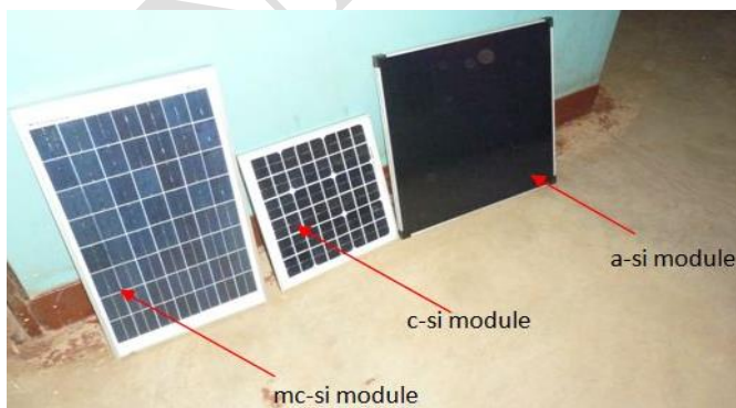
Figure 1. The PV modules of different technologies used in this study.
