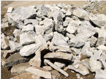
Step 1: Demolished concrete collection stone
