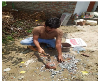
Step 2: Manual crushing
