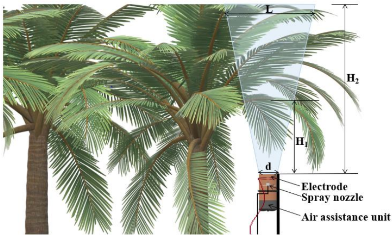
Figure 1. Air displacement diagram of the electrostatic sprayer for coconut palms
