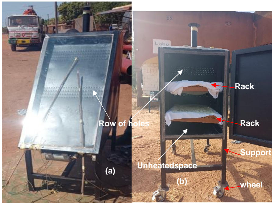
Fig.6Dryerbuilt in instrumentation
