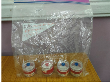
Plate 5: Collected filter cassettes sealed in Ziploc bag after the sampling period
