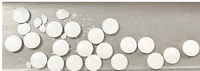
Figure 1: Tablet capping observed in formulation 1
