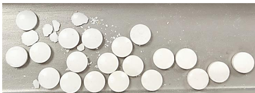
Figure 1: Tablet capping observed in formulation 1
