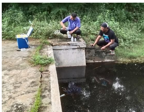
Figure 2. Leachate Sampling for Quality Standard Testing
