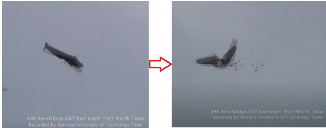
Fig.1 - Flutter during one flight demonstration – unmanned aircraft (Saemeil, 2007).
