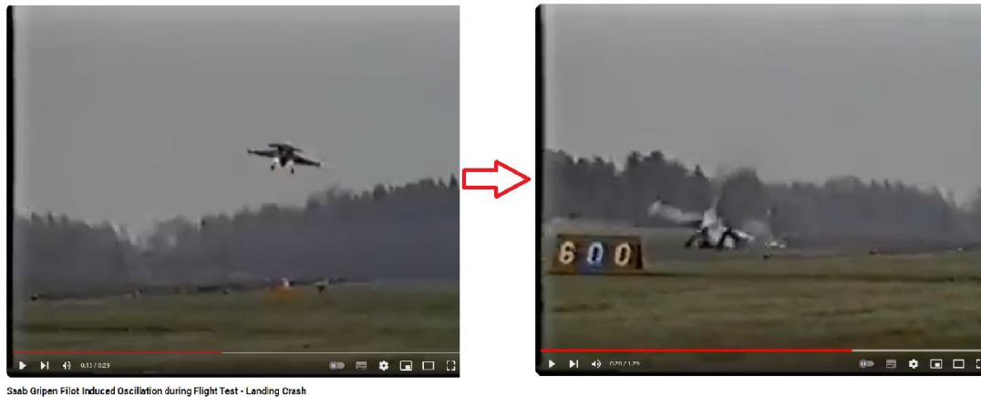
Fig. 4 – Saab Gripen pilot induced oscillation (MultiplyLeadership, 2012).
