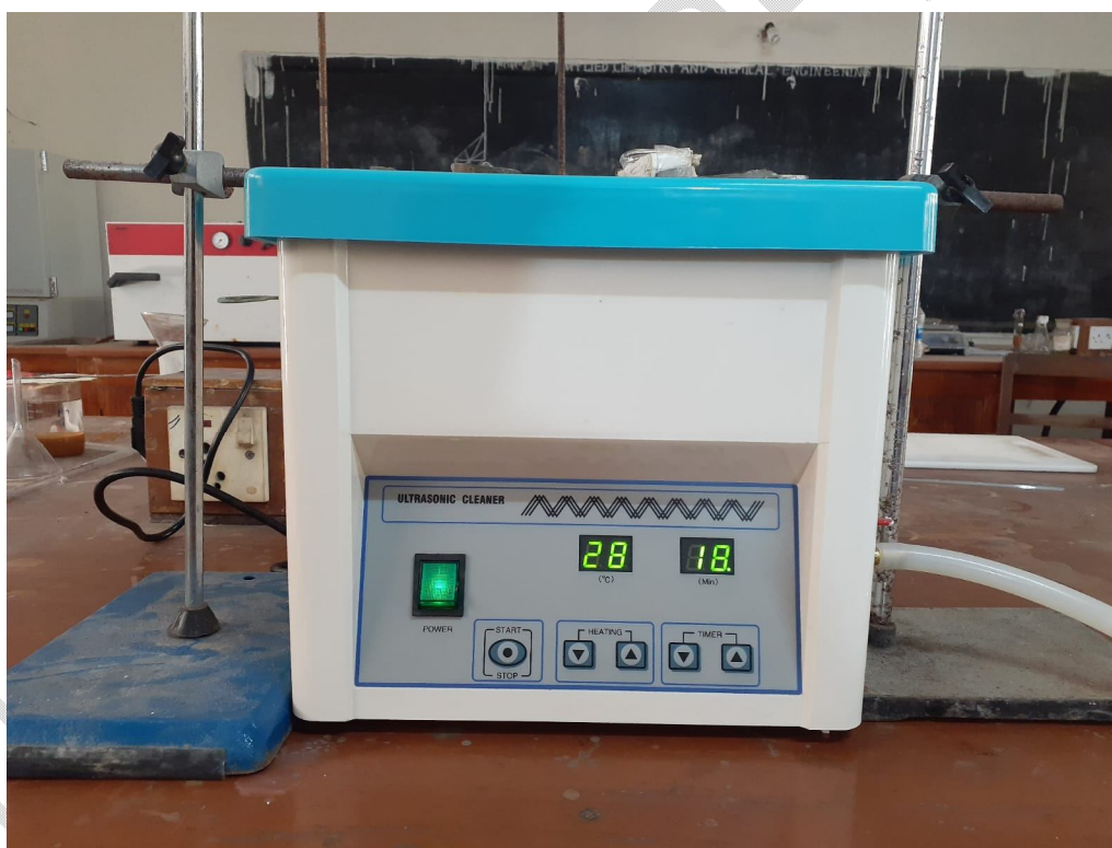
Fig. 1: Sonicator bath used in sonochemical degradation.
