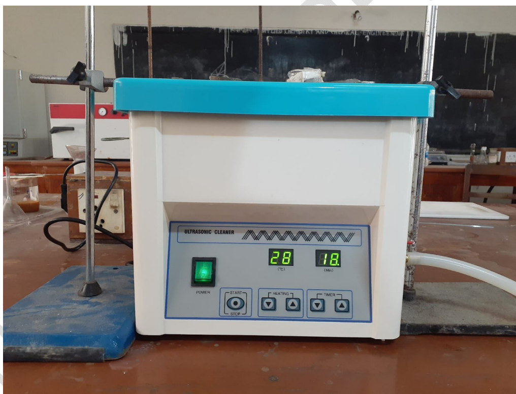
Fig. 1: Sonicator bath used in sonochemical degradation.
