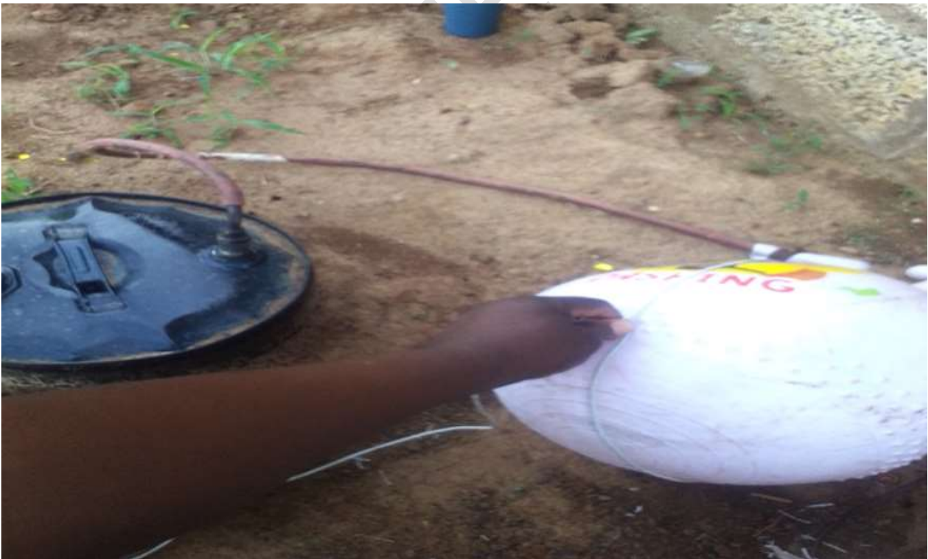
Fig 1. Shows a Metallic Drum Bio digester and a balloon as biogas collection chamber
