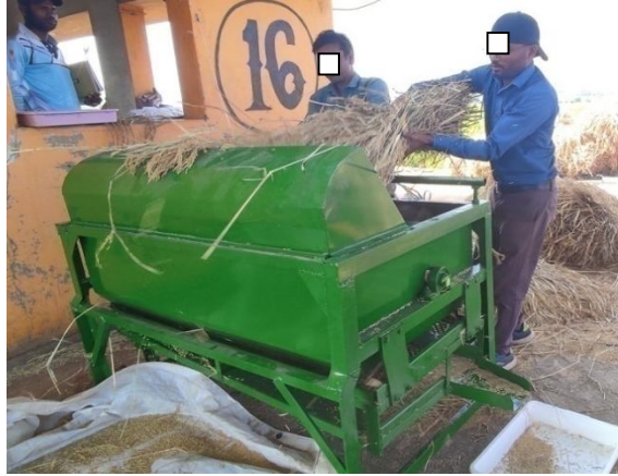
Fig.4 Power operated paddy drum thresher cum winnower (developed machine)
