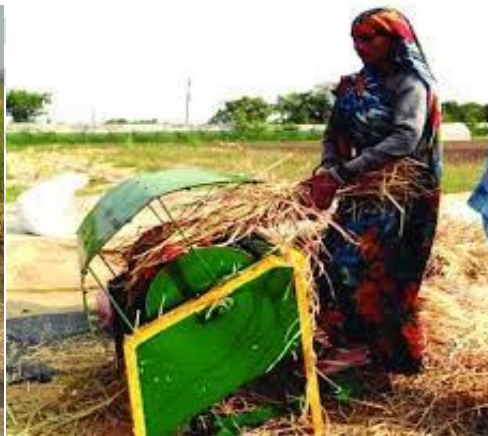
Fig.3 Pedal operated thresher
