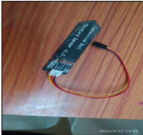
Plate 3 Capacitive soil moisture sensor v1.2
