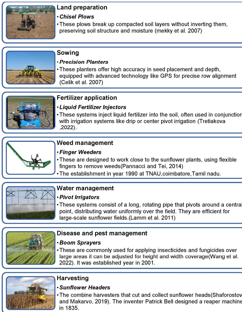
Fig.8.Flow chart of different machine's in sunflower cultivation
