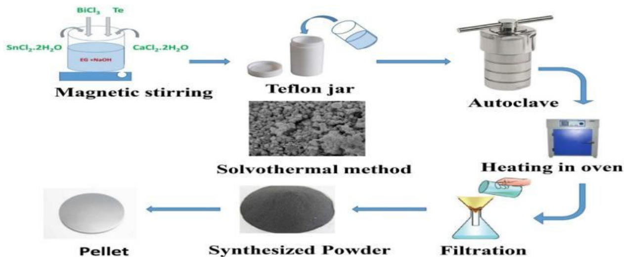
Fig 12. A schematic representation of the solvothermal synthesis. Reprinted with permission ref [88]. Copyright 2023, Springer
