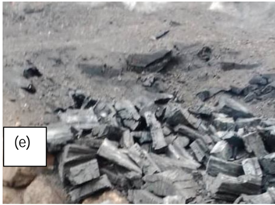
Figure 2: (a) Forest clearance/logs felled for charcoal production, (b) logs split to desirable sizes (c) splitted logs arranged in the earth pit kiln (d) earth pit kiln are covered by stones at the side and earth on top (e) earth pit kiln opened at the side of stones to exposed ready combusted charcoal (f) bagged charcoal, transported from forest to market
