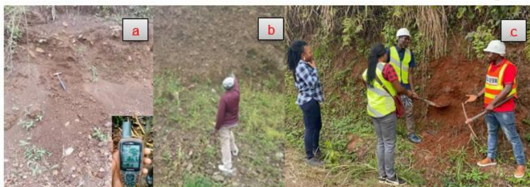
Fig.3.Field survey and sample collection showing: a. GPS Points recording and marking of outcrops,b. geologic description &c. sample collection
