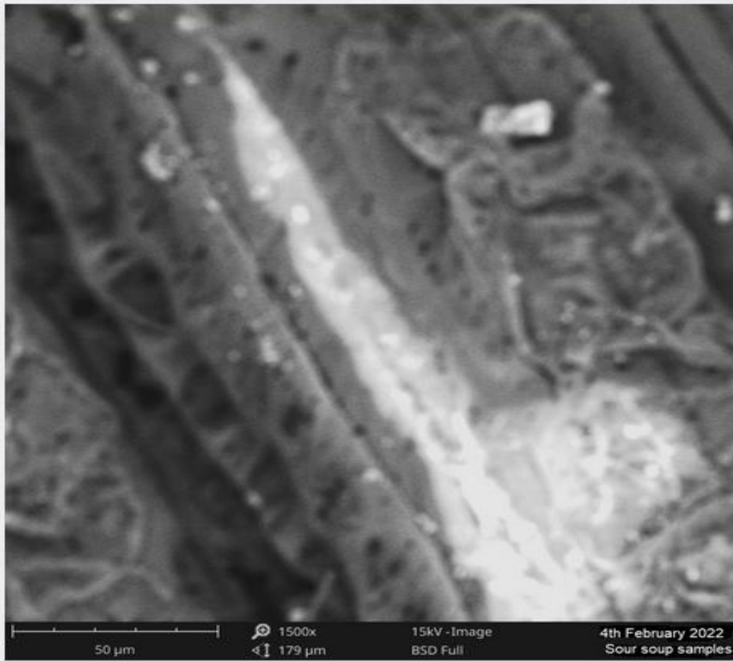
Figure 4: Scanning electron microphotograph of the biosynthesized silver nanoparticle (1500x magnification)
