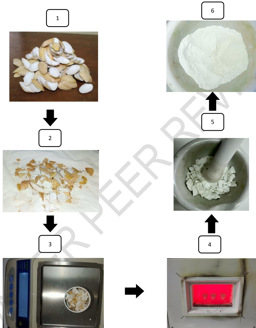
Figure 1. Steps of calcination of batik shellfish shells
