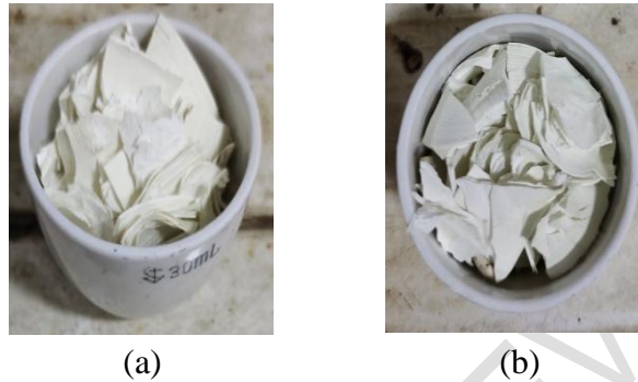
Figure 2. Powder resulting from the 8-hour calcination of batik shellfish shells. (a) At a temperature of 800°C. (b) At a temperature of 900°C.
