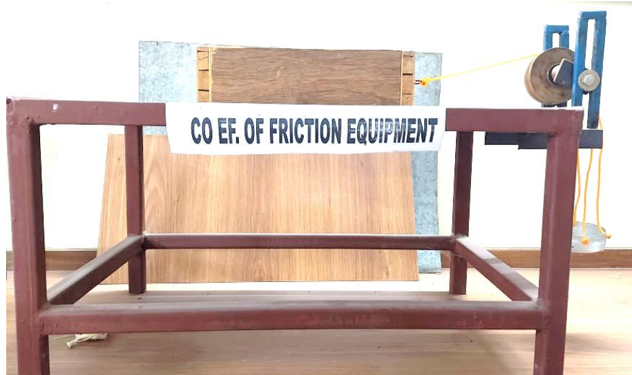
Figure 4. Measurement of coefficient of friction w.r.t. different materials
