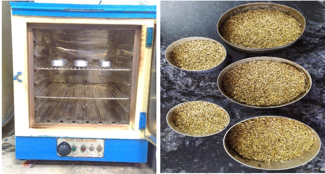
Figure 1. Measurement of moisture content through oven drying
