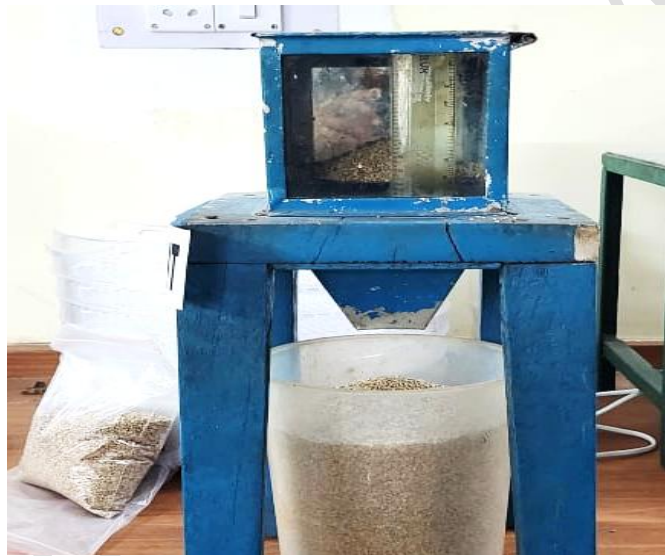
Figure 3. Measurement of Angle of Repose
