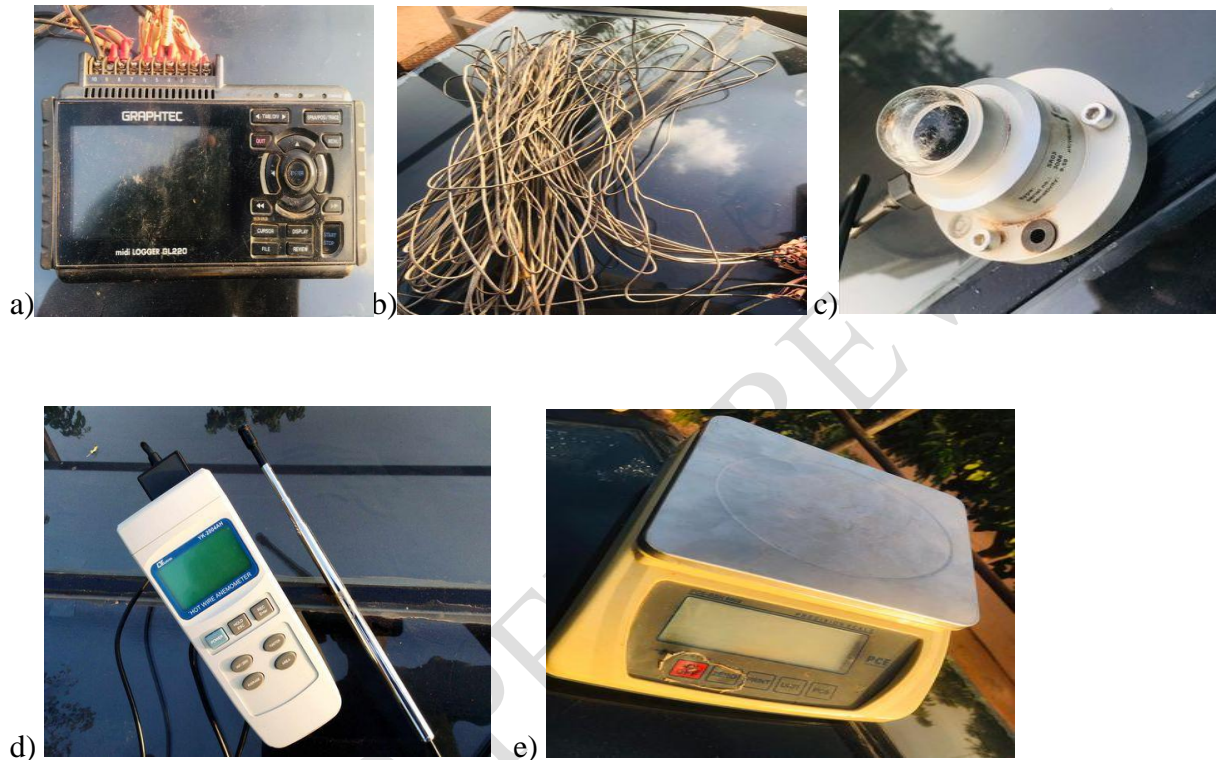
Figure 2: datalogger (a), thermocouples (b), pyranometer (c), anemometer (d), electronic scale (e)
