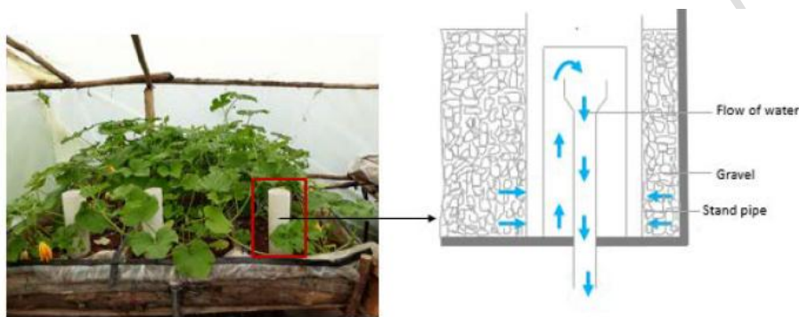
Fig. 2. Schematic layout of a hydroponic unit with a bell siphon
