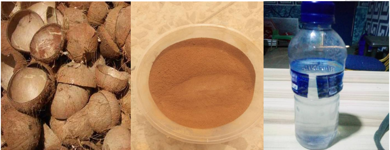
Figure 1 – photos of raw and crush coconut husk before activation and produced water sample
