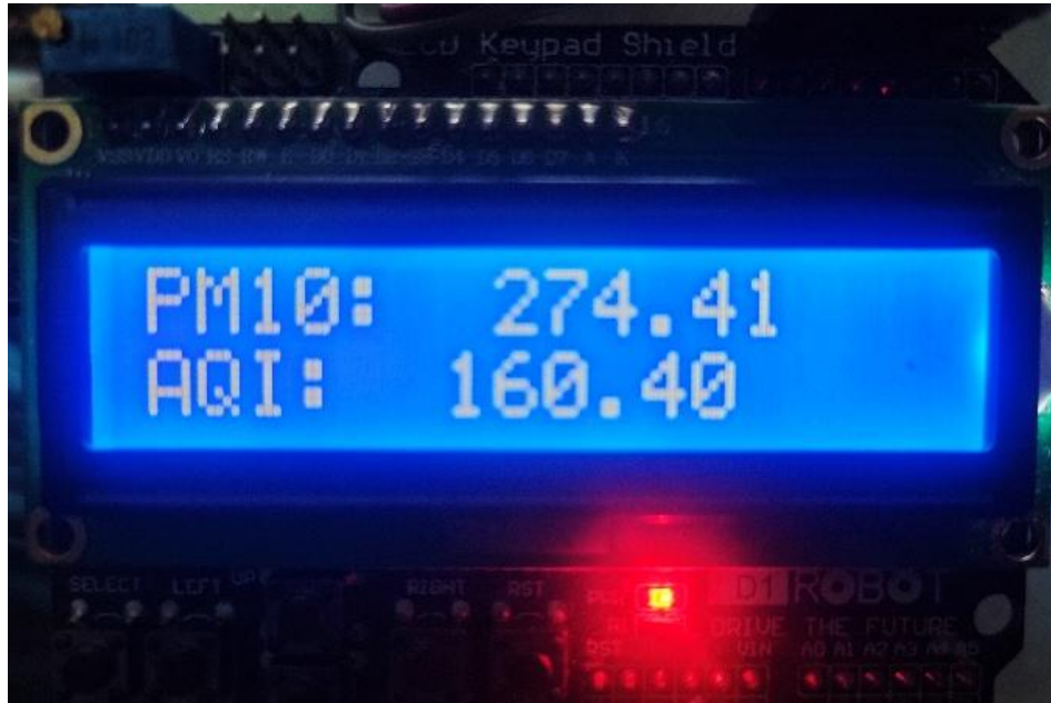
Fig.8.Experimental AQI data is displayed in real-time on the LCD screen with a red LED indicator.
