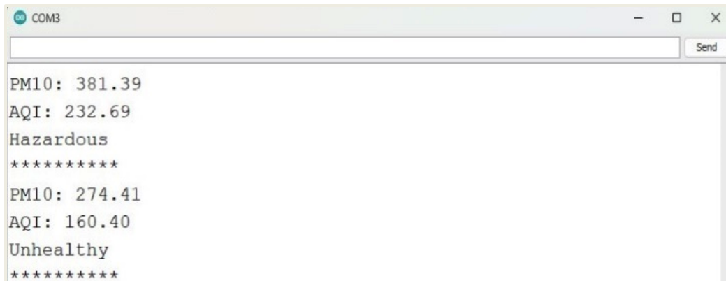
Fig.9.Experimental AQI data is displayed in real-time on the serial monitor of the Arduino IDE.
